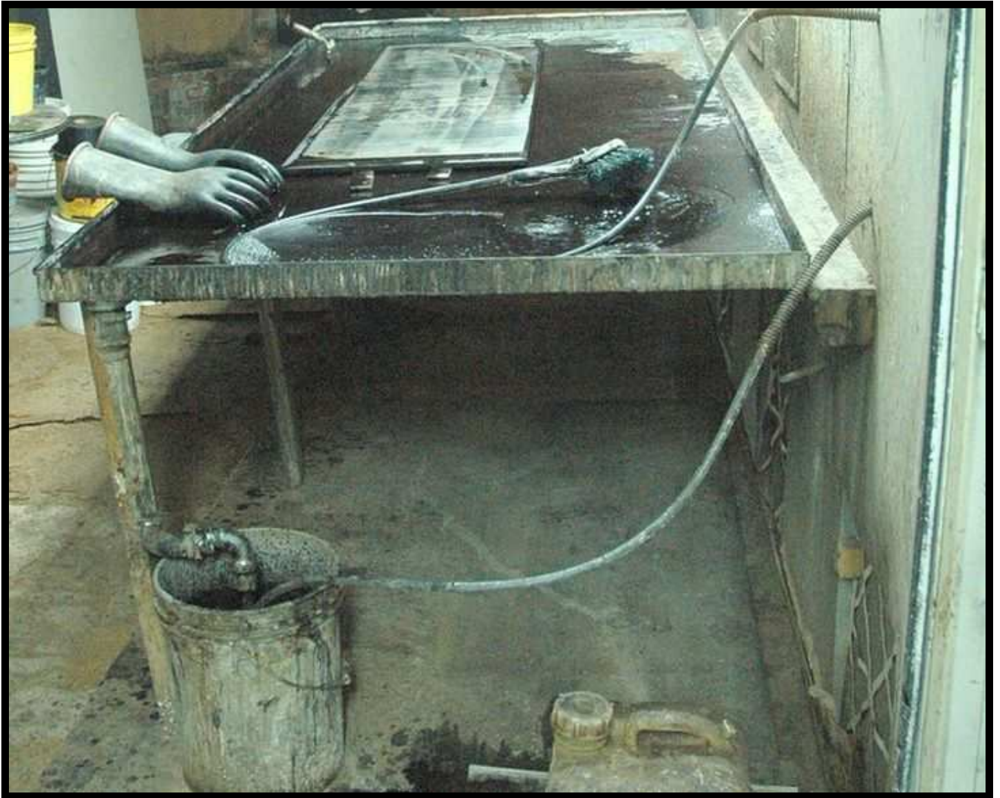
Strip room with section of the top having the old finish removed.
