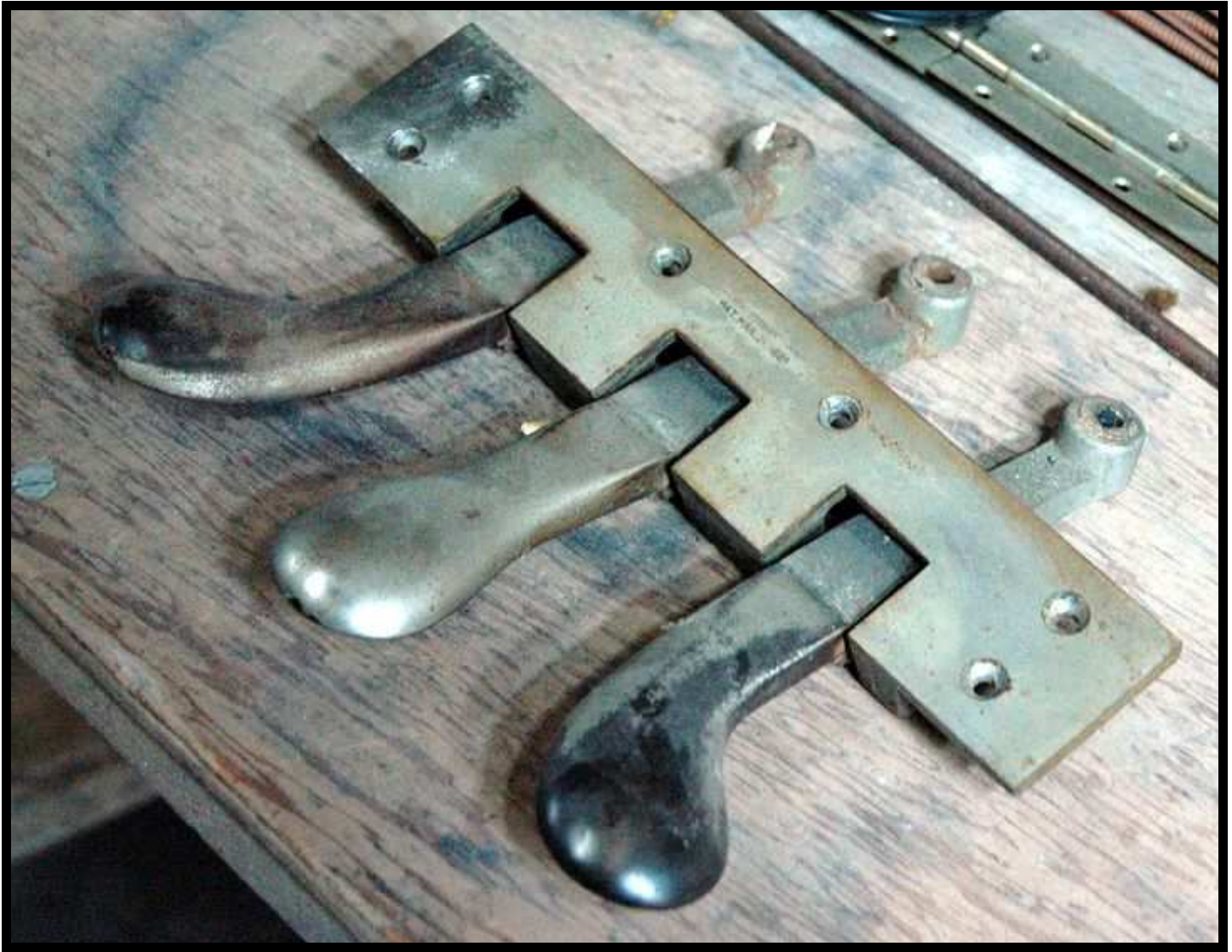
Additional restoration items: Pedals and pedal plate, prior to being sent to replating service for new chrome.
