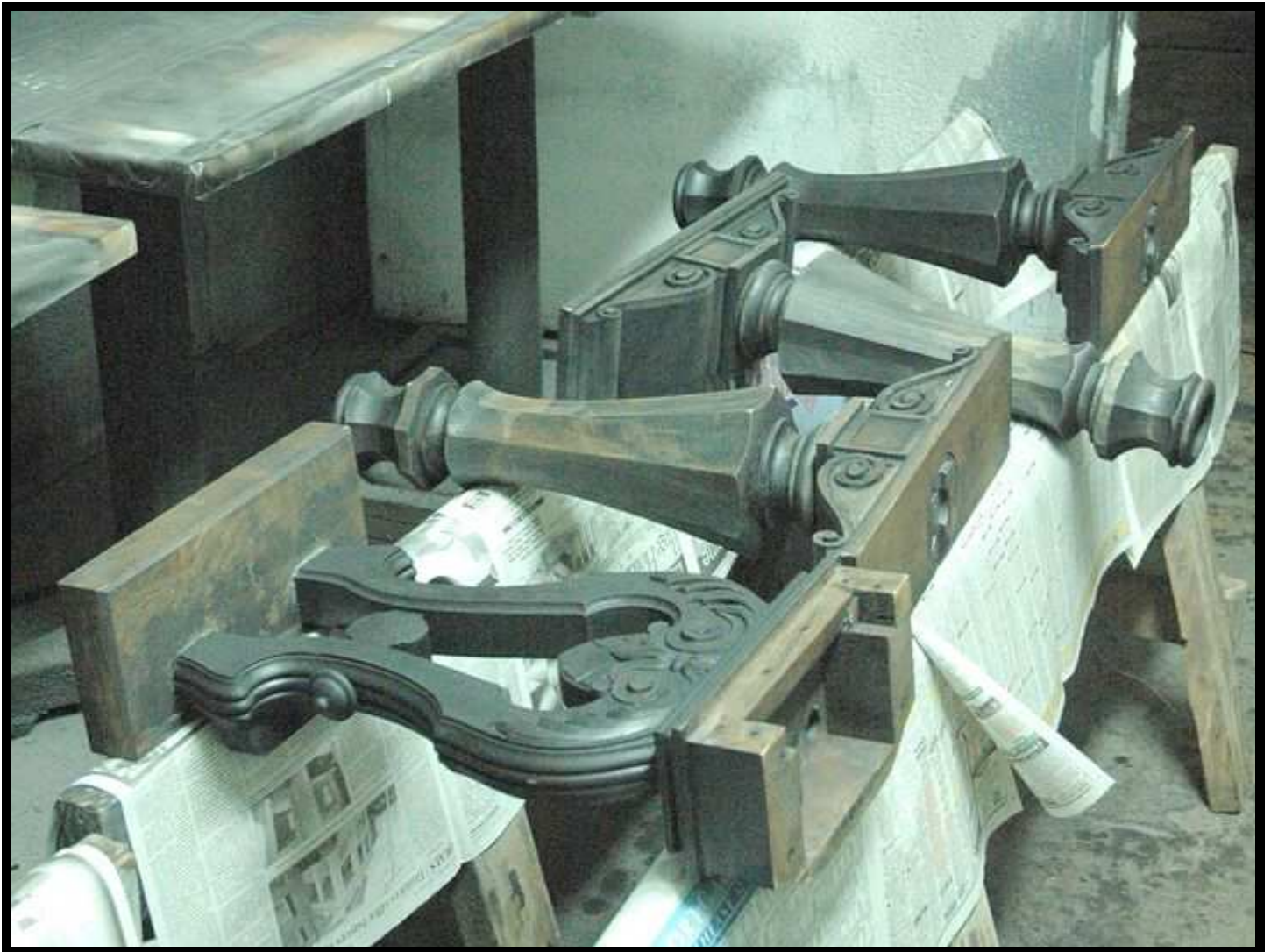
Piano legs and lyre after stripping. Next step is rinsing with a special solvent to remove all residue, prior to refinishing with the same steps shown for the piano casing.
